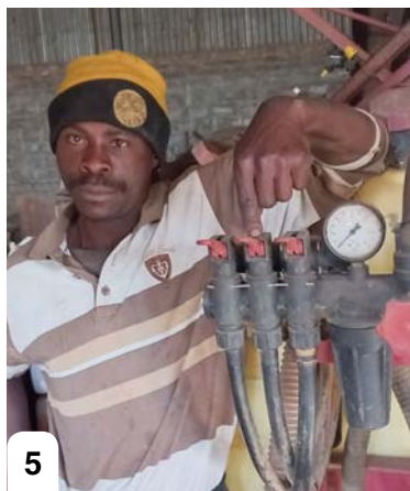
5 Replace or repair the control valve if it is not working properly.
