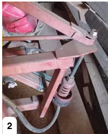
2 Lubricate all lubrication points especially the hinges of the spray beams.
