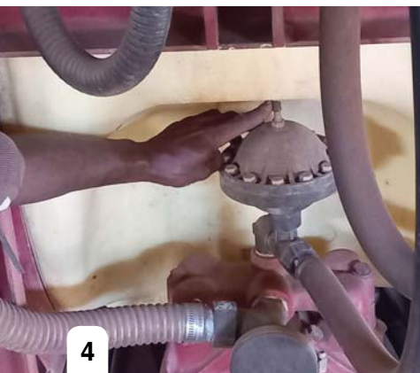
4 Looking for leaks on the pipes and fittings when the sprayer is working and when the valves are closed is important.
