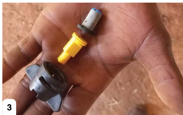
3 After flushing out the nozzles, reclean all filters and nozzles.
