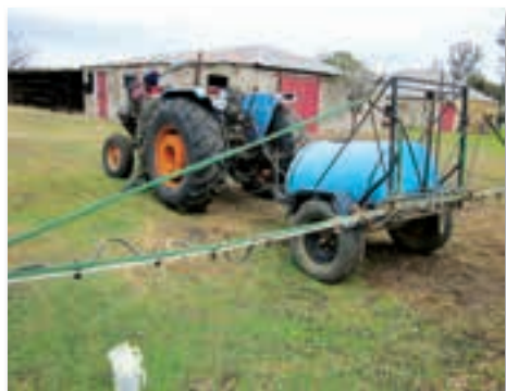
A boom sprayer which is used for chemical weed control.
