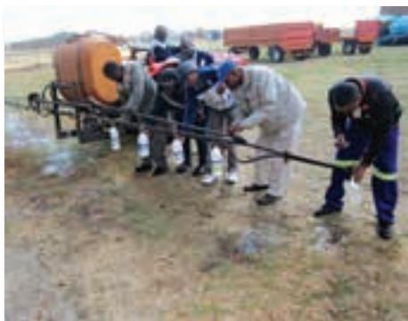
The calibration of a boom sprayer is very important to ensure the correct application rate of chemicals.
