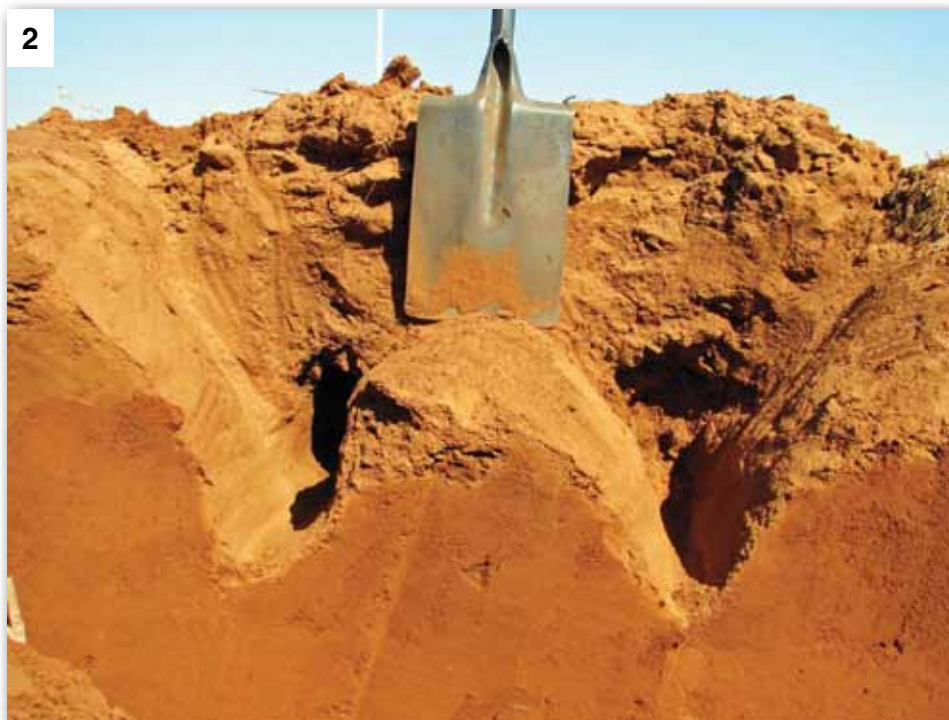
The operation of an implement can be seen clearly when a profile hole is dug where the implement has finished working.
