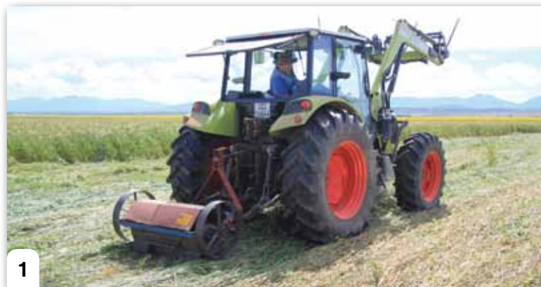
1 An example of a crimping roller.
