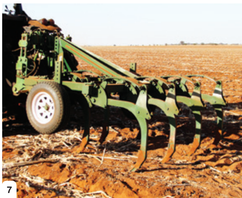
A chisel plough for compacted zones within 250 mm of the surface. Photo: Martiens du Plessis
