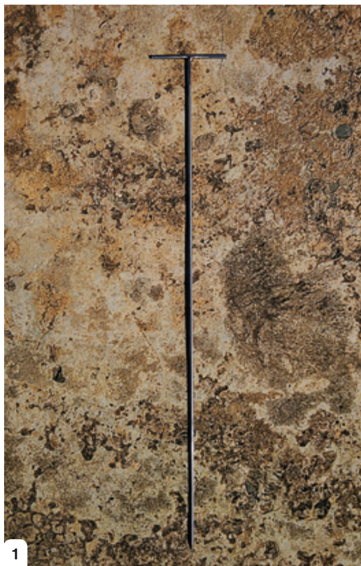
A home-made device for tracing compacted layers. Photo: Rianto van Antwerpen
