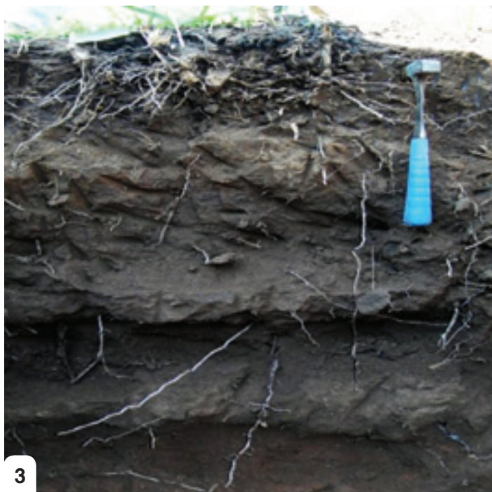
Three consecutive compacted layers in a field of sugar cane. Photo: Rianto van Antwerpen
