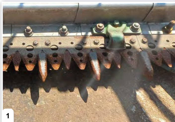
1 The cutter bar – with knives, guards and hold-down clips.
