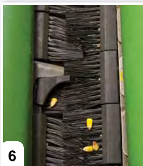
The new-generation replacement gathering chain.
