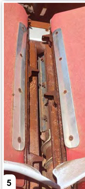
A maize header with the deck plates, gathering chain and snapper rollers clearly visible.
