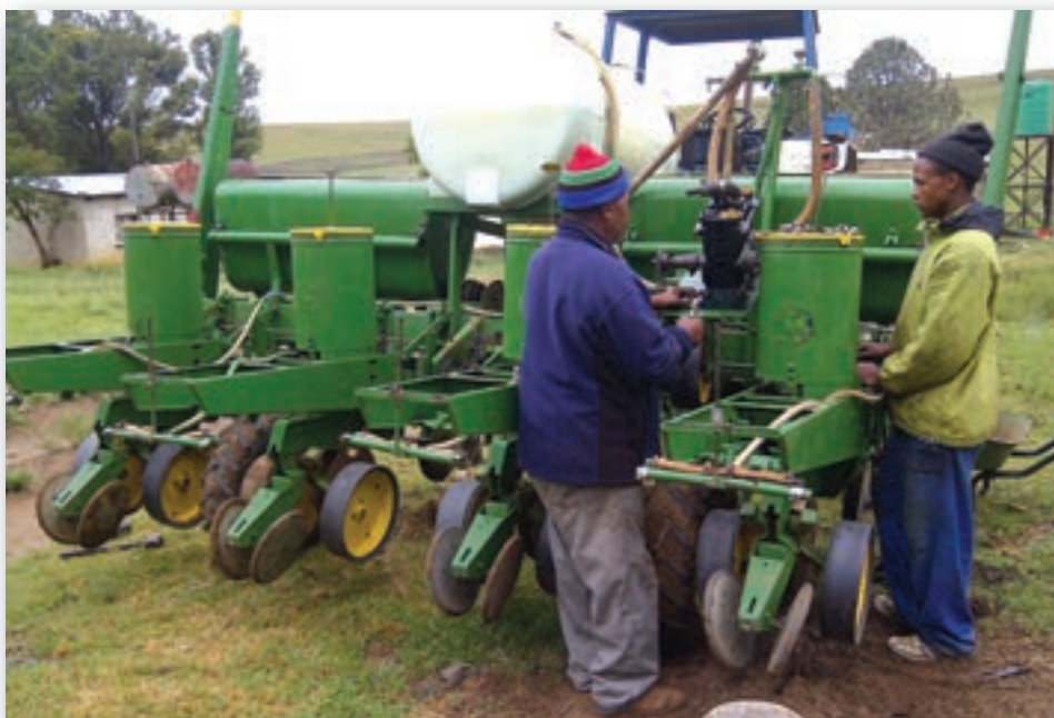
Ensure that all moving parts are turning and rotating freely with no resistance.
