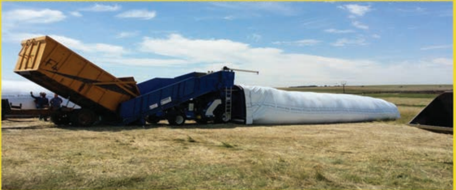
SELF-POWERED AND SELF-PROPELLED SILAGE BAGGING MACHINE
