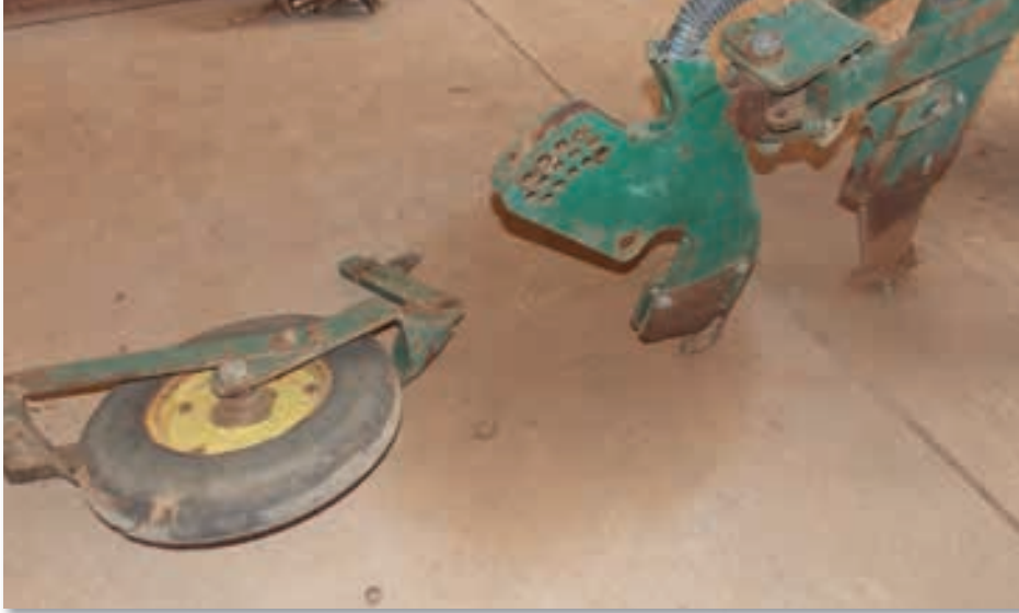
The wheel is removed to replace wheel bearings that are worn.
