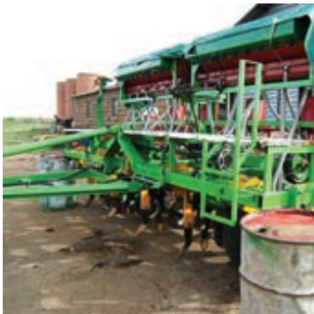
Photo 1: Home-built Agrico chisel-plough frame with (yellow) tine units by Alpha Engineering in Swellendam.
