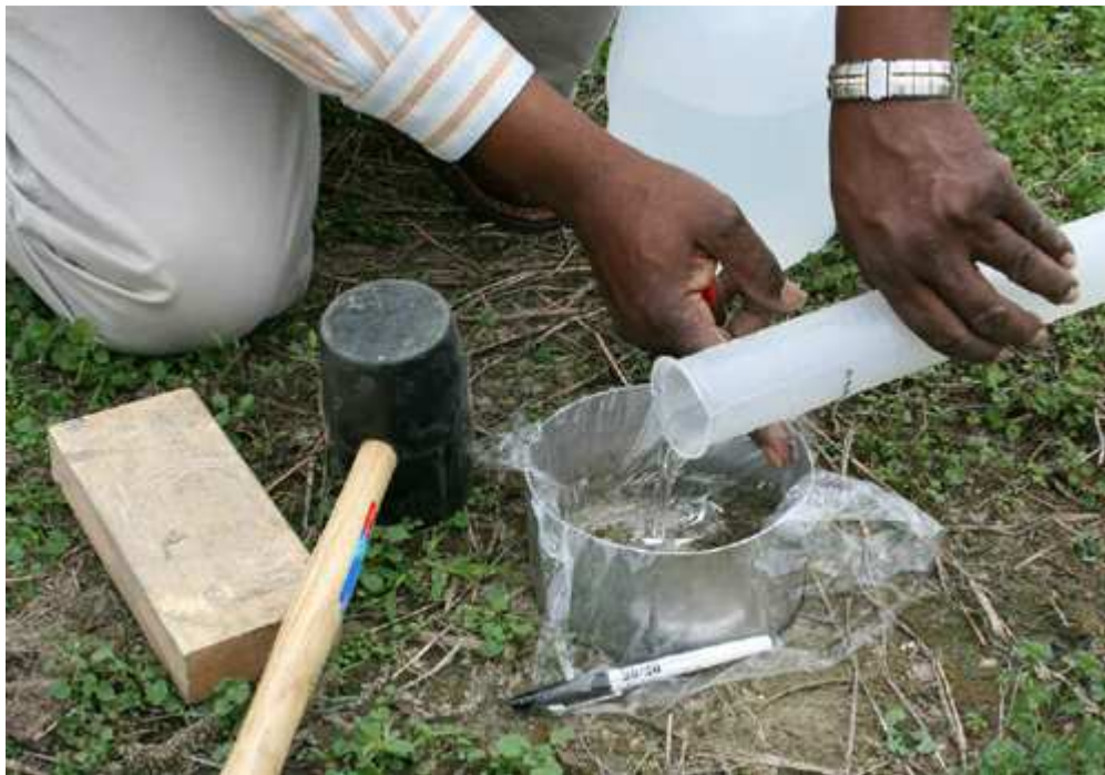
Figure 8.3.3. Infiltration test being performed.
