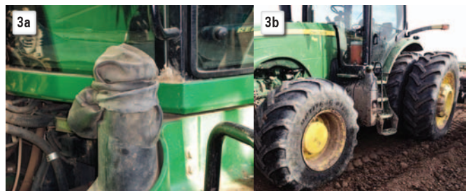
▲ 3a and 3b: Improper maintenance and sealing of equipment fuel tanks. With Tier 4 engines, cleanliness of the diesel exhaust fluid (DEF) dosing module is also critical to ensure proper operation of equipment.
