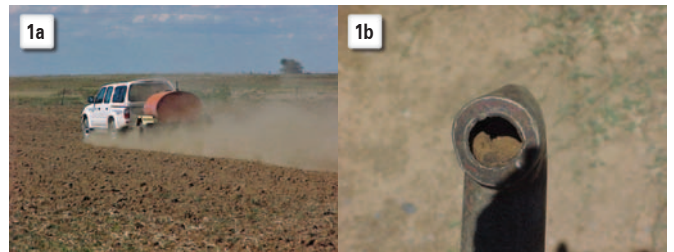
▲ 1a and 1b: The way fuel is transported to the field on dusty roads, with the breather of the mobile fuel cart being just an open pipe and with the outlet hose and nozzle not covered, increases the contamination of the fuel.
