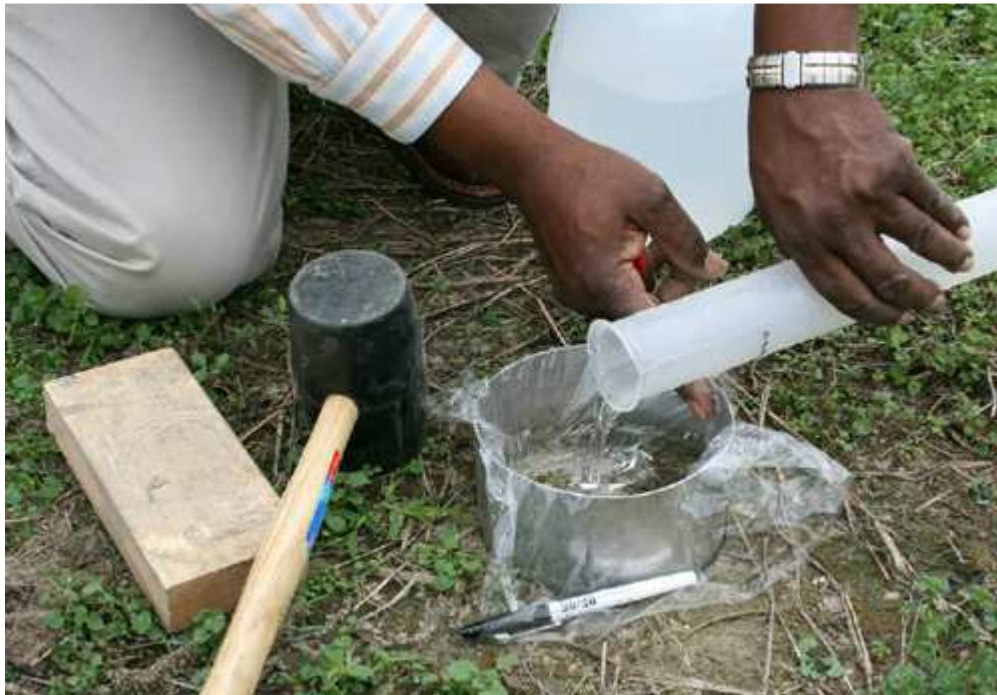
Figure 3.21. Infiltration test being performed
