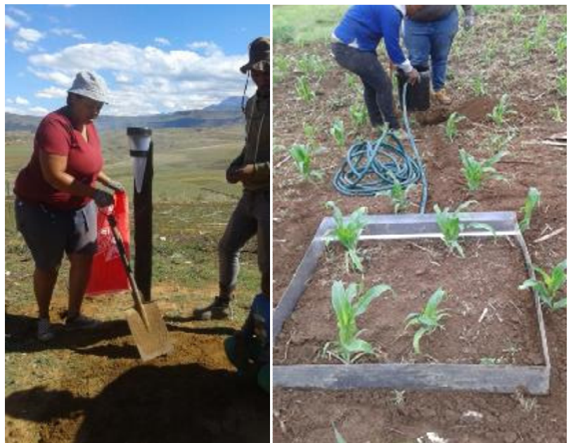
Figure 41: Left-MDF team installing rain gauge at Mam Ntombakhe Zikode's homestead and Right- MDF team installing Run-off plots in Mrs. Zikode's trial.
