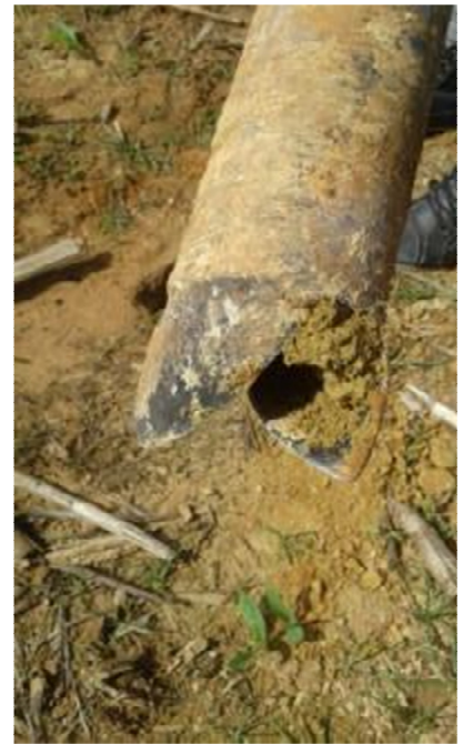
Figure 5: A gravimetric soil sample taken at Ntombakhe's trial plot, showing the clay and shale parent material in this 30cm depth sample
