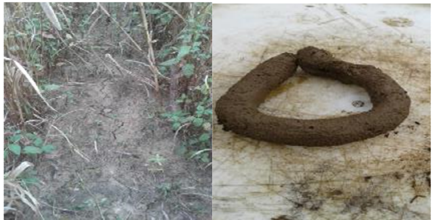
Figure 3: Right: Crusting and cracking in the soil shown in Dlezakhe Hlongwane's field and Far Right: A soil sausage made from his soil indicting the high clay content.
