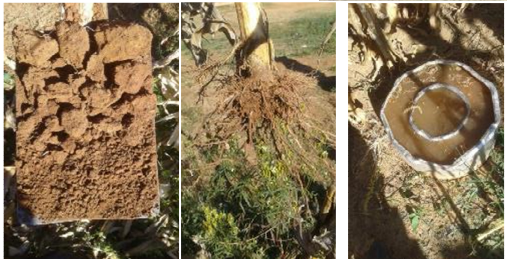
Figure 6: From Left to Right: A spade of her soil graded to show large clods but little structural integrity; An example of root size and depth of one of her maize plant - showing quite shallow rooting and the double ring infiltrometer set up for readings. The walls of the rings are quite battered due to extreme difficulty of getting the rings into the soil
