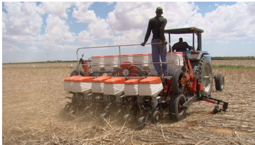
Photo 5.1: A Jumil planter in action on the trials at Humanskraal 2017/2018 demonstrating its ability to plant successfully through crop residue.
